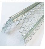
USE: It is galvanized steel and has full 3-1/8" flanges. It is easily adjusted for plaster depth on columns and is ideal for structural tile corners with rough masonry. Double X Corner Bead has perforated stiffening ribs along the expanded flanges.
