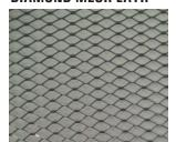
USE: Manufactured by slitting and stretching galvanized steel to form small openings to allow the keying of plaster so it will bond to the lath. Diamond Mesh Lath can be bent easily to create curved surfaces. SIZE:
