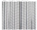
USE: Superior spanning characteristics over common expanded metal laths, suited for horizontal applications such as ceilings and soffits. Its 3/8" deep ribbed configuration is a self-furring feature. Designed for application on 24" on center. SIZE:
