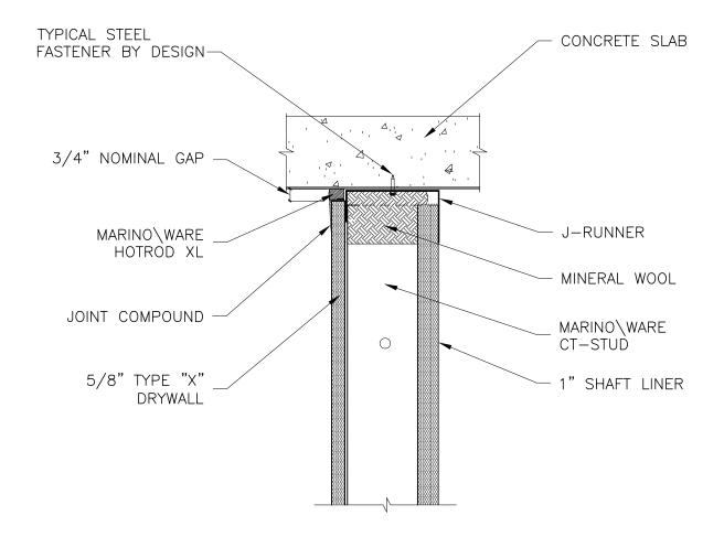
HW-D-0625 1 & 2 HR SHAFTWALL, CONCRETE SLAB
