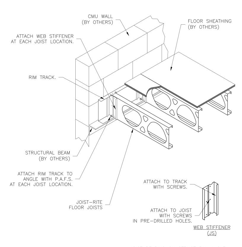
JOIST BEARING ON STRUCTURAL ANGLE ATTACHED TO CMU WALL
